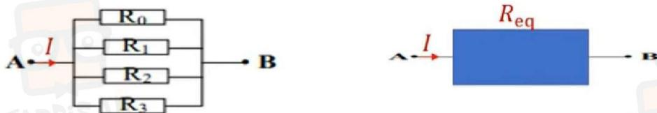
$$\frac{1}{R_{eq}} = \frac{1}{R_0} + \frac{1}{R_1} + \frac{1}{R_2} + \frac{1}{R_3} = \frac{1}{4,5} + \frac{1}{2} + \frac{1}{3} + \frac{1}{2,5} = 1,455 \quad R_{eq} = \frac{1}{1,455} = 0,69\Omega$$
